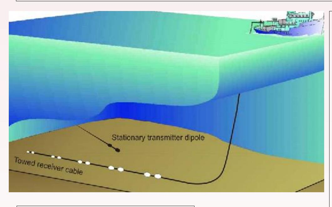
This is a deep-sea towed transmitter system which is known as DASI. The DASI (Deep-towed Active Source Instrument) is a system used for controlled-source electromagnetic sounding in marine environments.
