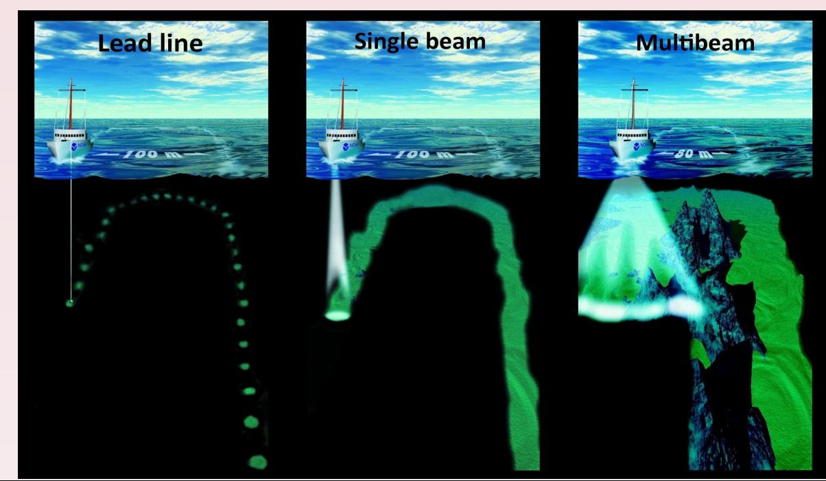
A side scanner is a type of single beam sonar and since it is only one beam transducer it can only replicate and produce a 2D image of return signals that has bounced off objects or the ocean floor. A multibeam sonar system uses multiple transducers, mounted to the ship's hull and pointing at different angles on either side of the ship and uses the return signals to create a 3D bathymetric map of the ocean floor.
